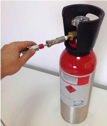
3. Purge air/hydrogen quantities out of hose connected to hydrogen source by the mean of a compatible original H2planet refilling kit/H2planet Hy-Flow or Hy-PEM XP connection kit or with compatible Swagelok QC4 connectors. Please push on top of stem-male quick connection kit for a few seconds according to relevant instructions in order to purge possible contaminating gases such as air/nitrogen or other. You will hear a pressure coming out of hose.
